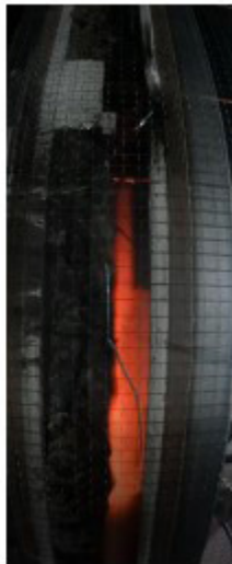
Flames reach cavity barrier t=80s
