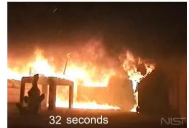
32 seconds Room fills with hot smoke; remote items ignite
